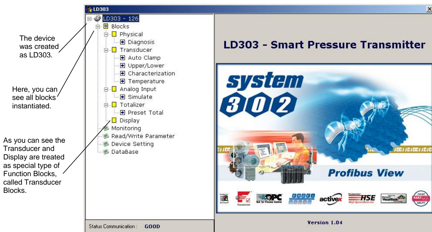
Figure 3.2 - Function and Transducers Blocks – Profibus View
