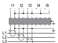
For a 3-phase 3-wire system, the meter measures the residual current for Ground at I4.
