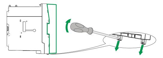
2. Holding the meter firmly, swing it outwards and pull slightly upwards to detach it from the top retaining hooks.
