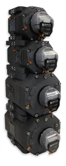
model Rotary Gas Meter is a special designed magnetic coupling where one part is fitted inside the meter body and the associated part is placed in the read-out unit. The read-out unit can either be a mechanical index or an electronic index, with or without volume conversion and communication functions.
