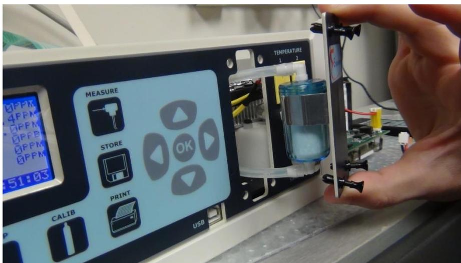
The condensation filter is typically replaced much less frequently than the line filter and should be replaced if it becomes saturated with water. This filter is accessed by opening up the analyzer. More details can be found in the Maintenance section (Chapter 12) of the complete E8500 Plus operating manual.
