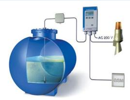
Monitoring of the level in an outdoor rain water tank. A combined alarm light and horn is connected in the vicinity of the tank; TankControl 10 is installed inside the building. It is also possible to connect a float switch to monitor for backflow from the drain. The system can be extended by a GSM-based event reporting system.
