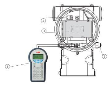
1 Handheld communicator | 2 External ground termination point | 3 Battery | 4 Fast connection for harvesting unit
