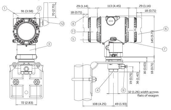
1 Adjustments | 2 Identification plate | 3 Certification plate | 4 Process connection | 5 Terminal side | 6 L1 and L5 integral display housing | (7) Electronic side (8) Space for cover removal (9) Drain/vent valve (11) Battery housing of WirelessHART version (12) Antenna of WirelessHART version
