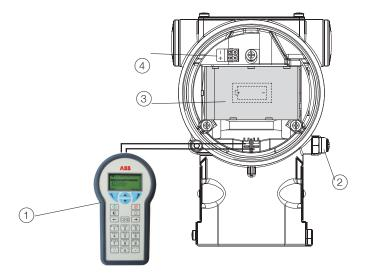
1 Handheld communicator | 2 External ground termination point | 3 Battery | 4 Fast connection for harvesting unit
