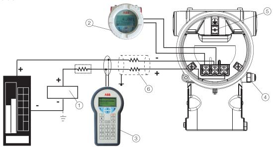
HART hand-held communicator may be connected at any wiring termination point in the loop, providing the minimum resistance is 250 ohm. If this is less than 250 ohm, additional resistance should be added to allow communications. Maximum voltage drop on external remote indicator is 0.7 V DC.
