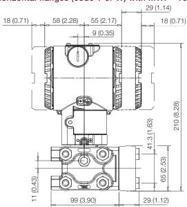
Process connection, gasket groove and gaskets are in accordance with IEC 61518.
