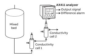
Dual input comparator for critical measurements
