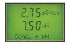
Simultaneous conductivity and pH measurement
