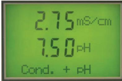
Simultaneous conductivity and pH measurement
